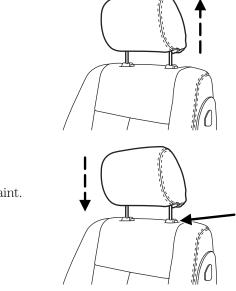
3. Lower the head restraint by pressing and holding the guide sleeve adjust/release button and pushing down on the head restraint.
